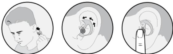
1. Starting with the EarLock® retention ring oriented slightly backward, rotate the earplug forward while inserting the stem of the red-filtered EP3 into the right ear canal deep enough for the uppermost flange to seal. Fit the retention ring to the natural contour of the concha bowl surrounding the ear canal to lock the earplug in place.
